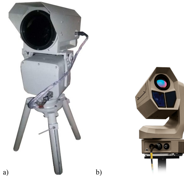
Fig. 25. Photo of two long range thermal imagers of similar operational range a)uncooled Sadad 102 thermal imager from Iran Electronics Industry [103] , b)cooled Ranger HDC from Teledyne-FLIR
