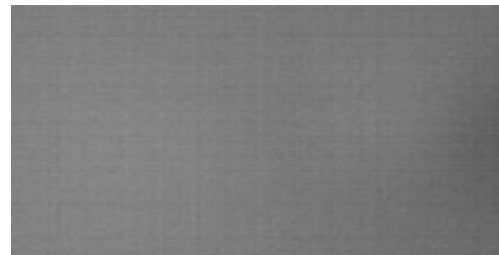
Fig. 8. Image of a large passive blackbody that fully fills the imager's FOV.
