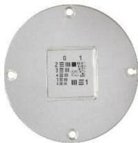
Fig. 17. Photo of USAF 1951 target of 100% contrast
