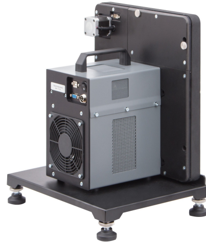
Fig. 14. Photo of MRW-8 rotary wheel with attached TCB-2D blackbody blackbody
