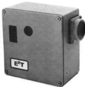
Fig. 3.3. Dualband narrow-band atmosphere pyrometer: DICHROMA manufactured by E 2 T ®
