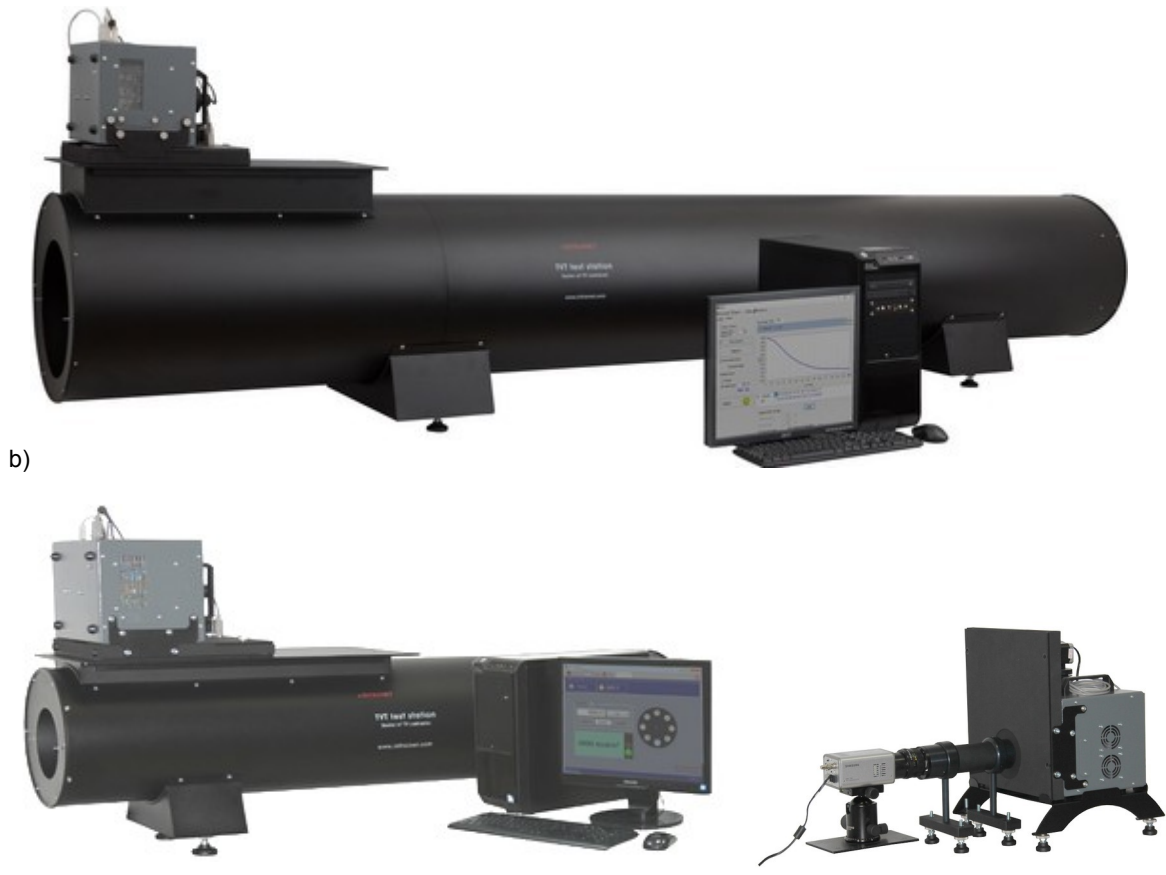
Fig. 1. Versions of TVT test system: a)TVT300 for testing long range VIS-NIR cameras, b)TVT150 in configuration for testing medium range VIS-NIR cameras, c) TVT150 in configuration for testing short range cameras (CCTV cameras)
