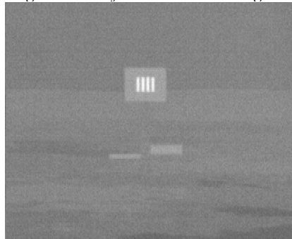
Fig. 2. Image of the TAFT set generated by the tested imager during MRTD measurements
