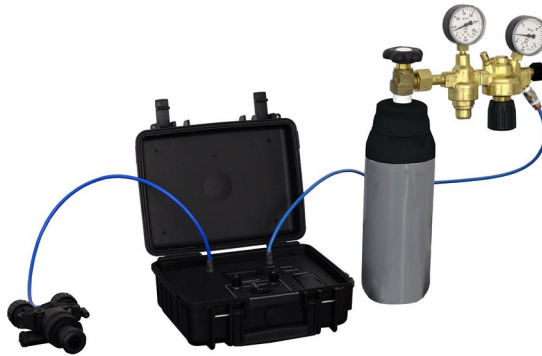
Fig. 1. Photo of the NPL purge-leak station
