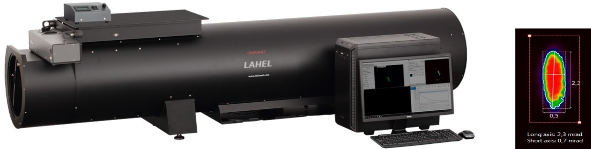
Fig. 1. LAHEL300 test system: a)photo, b)angular spatial intensity distribution of tested HEL
