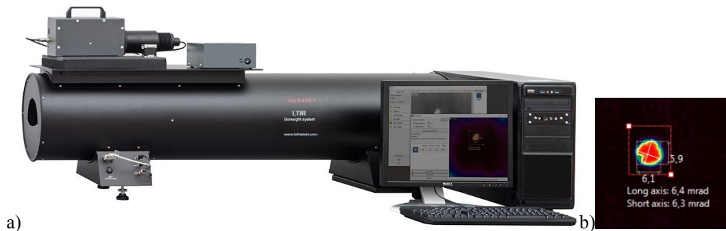
Fig. 1.LTIR test/boresight system: a)photo, b) exemplary measured spatial intensity profile
