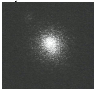
Fig.2. Image of illuminated field by laser illuminator of poor illumination uniformity
