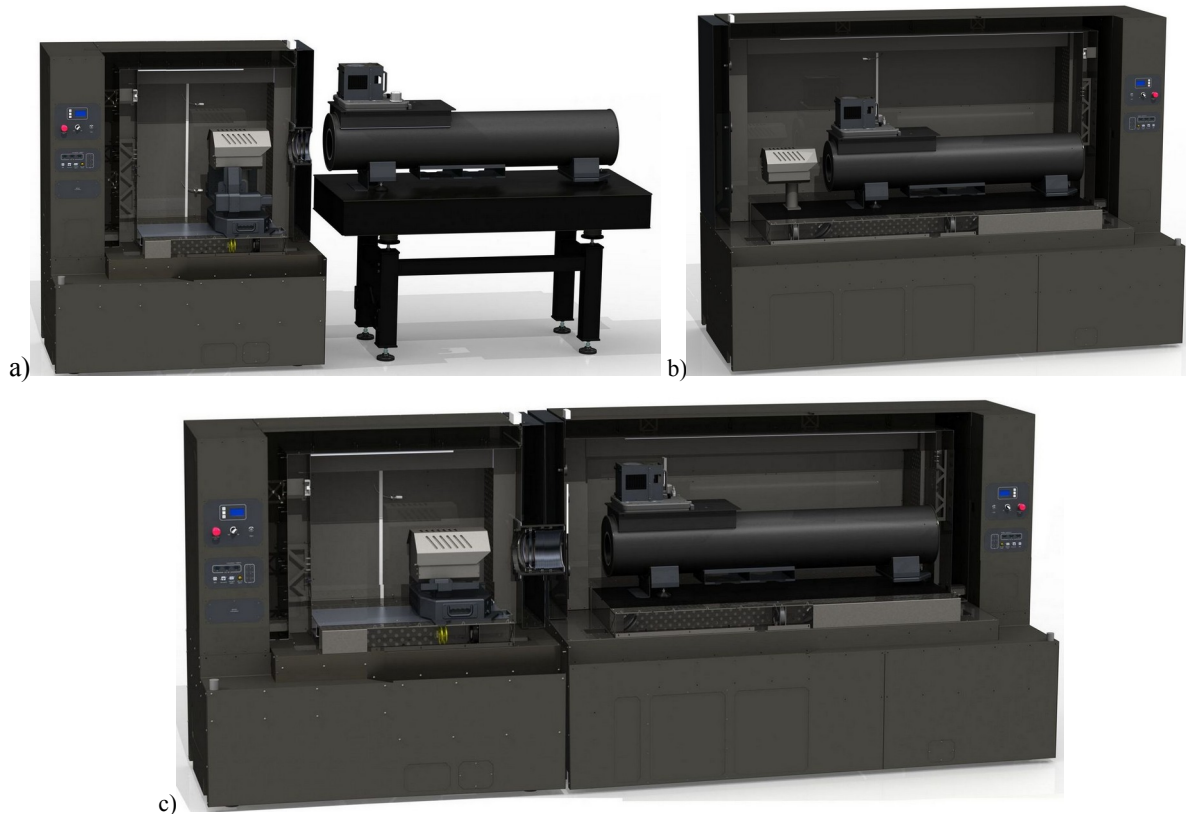
Fig. 1. Cross section of a)EXIR-1, b)EXIR-2 , c)EXIR-3 systems for testing thermal imagers at extreme conditions
