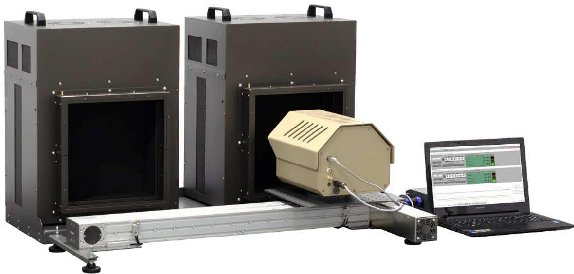
Fig.1. Photo of BNUC-12D-2TCB-TC set for 2 point NUC (including YLS
